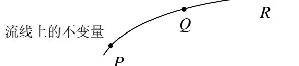
$$\text{静止流体: } v_1 = v_2 = 0, \text{ 伯努利方程} \rightarrow p_1 = p_2 + \rho g \underbrace{(y_2 - y_1)}_h$$
