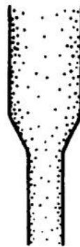
Schematic drawing of a cross section through a neck region of drawn polymers
